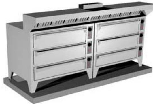
2. An eyebrow hood that will extend the full length of the oven with the inside edge of the hood overhang of the oven door opening(s) by at least 36-inches. Use the formula  $Q=60A$  to calculate minimum hood exhaust volume.
