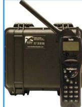
Larger offices may want to consider a fixed satellite phone unit, which can provide satellite-based telephone using an outside antenna and any analog phone. While somewhat more expensive than a handheld satellite phone, this system also requires a backup power supply and may therefore be of limited utility in worst-case scenarios.
